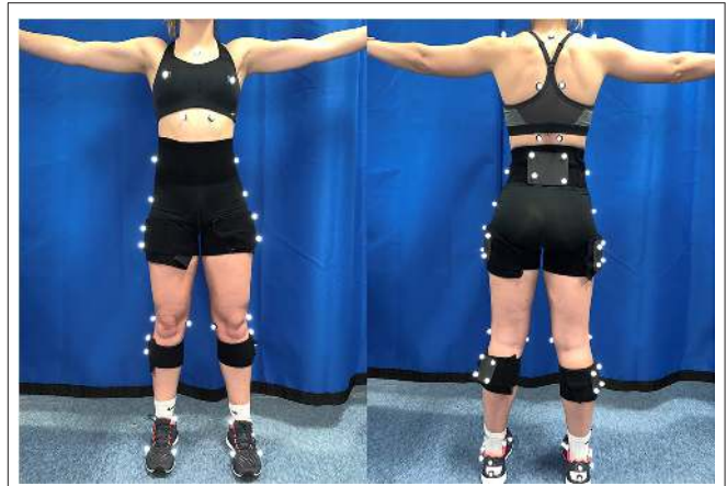
FIGURE 1 | Image of retroreflective marker locations used to define and trunk the skeleton including the trunk, pelvis, right and left thigh, shank and foot. Anatomical markers including the left and right iliac crests, greater trochanters, medial and lateral femoral epicondyles and medial and lateral malleoli as well as the first and fifth metatarsals were removed prior to dynamic testing.
