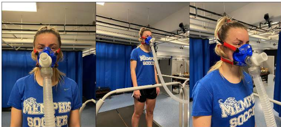
FIGURE 2 | Anterior and anterolateral views of the ParvoMedics TrueOne metabolic measurement system. Expired gases were collected from the participant via a face mask and plastic hose. A proper seal around the mouth and nose was confirmed by research staff prior to testing.
